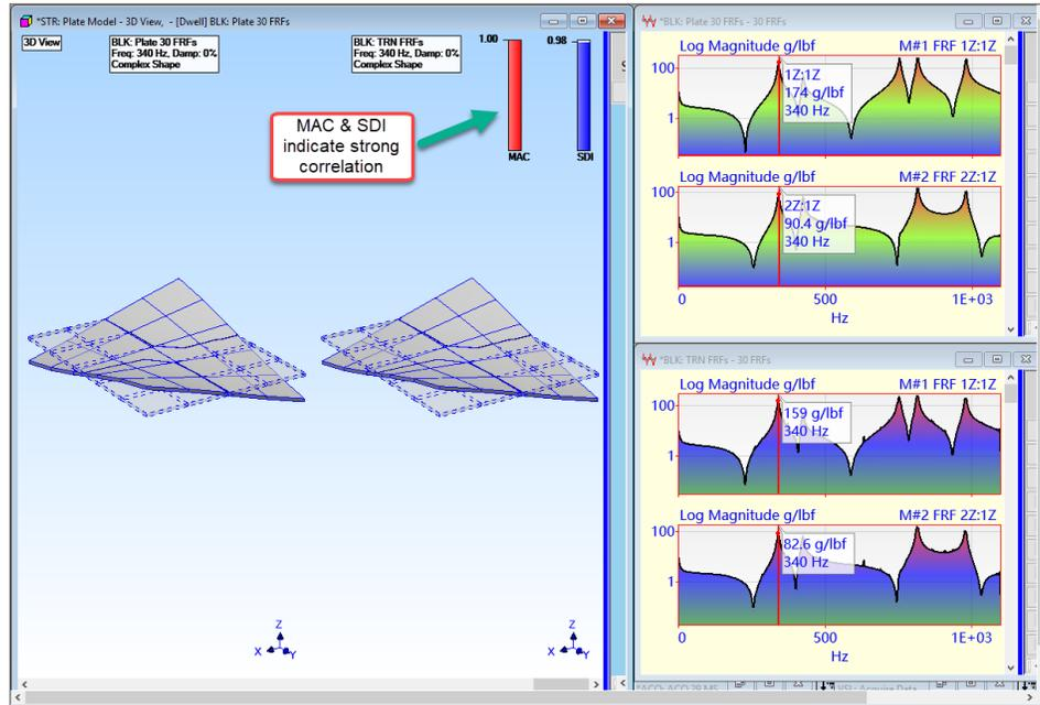
Drag the cursor to each resonance peak in the FRFs to display its ODS. Notice in the figure above that **MAC = 1** and the **SDI = 0.98** between the **340 Hz** ODS's in the two Data Blocks. MAC indicates the *co-linearity* between two shapes, and SDI measures the *difference* between two shapes. Both metrics indicate a strong correlation between the ODS's at the 340 Hz resonant peak.
