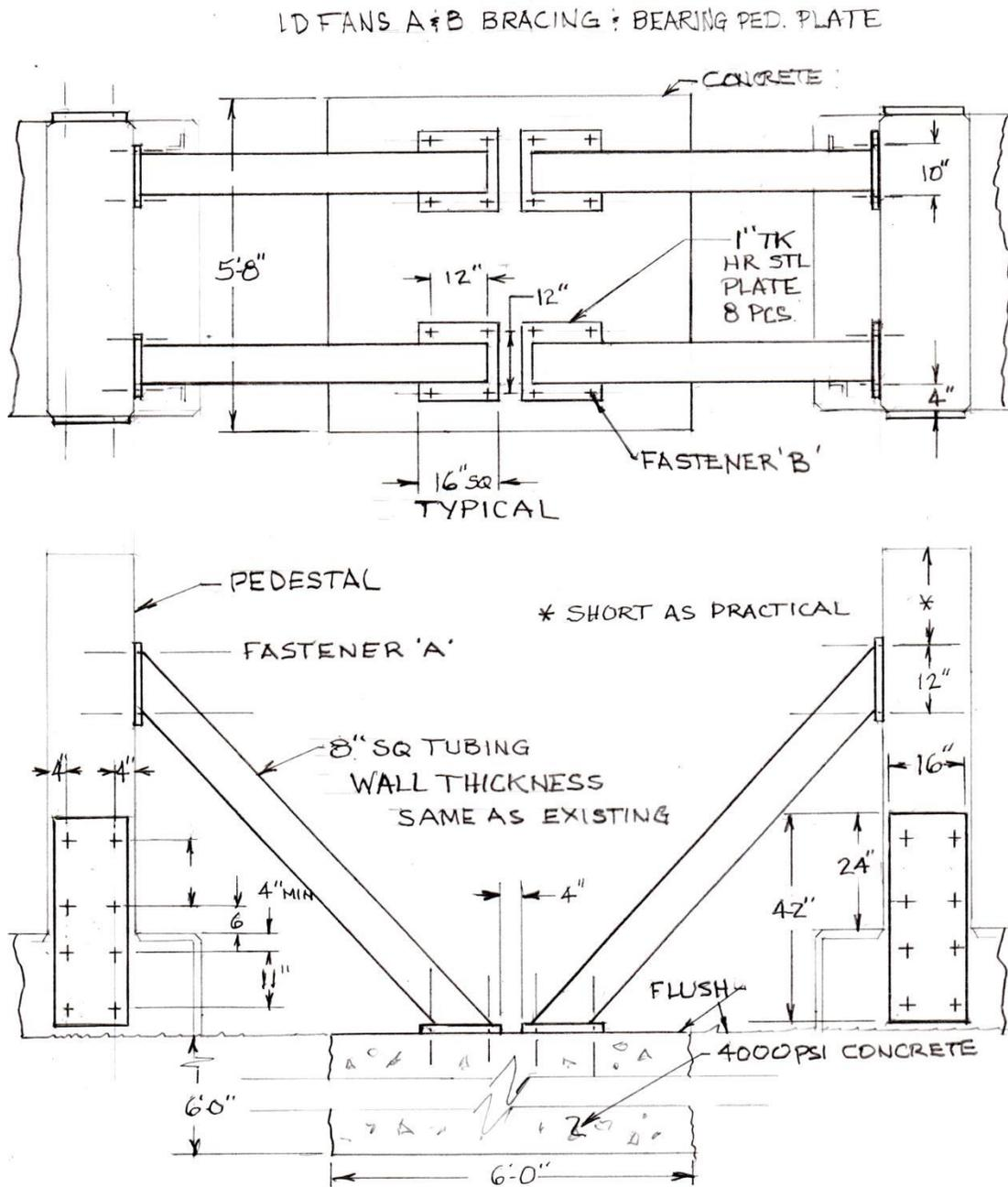
**Figure 40. ID Fans A & B Revised Bracing and Pedestal Plate Support.**
