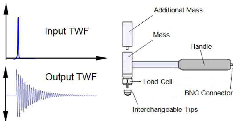
**Experimental Modal Test Instrument Setup Parameters**
