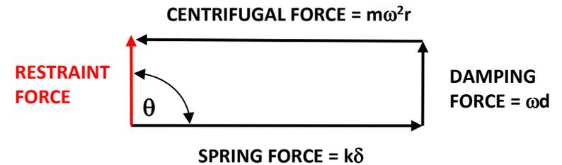
**AT RESONANCE: DAMPING CONTROLLED**
